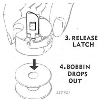
Fig. 14. Removing Bobbin from Case
